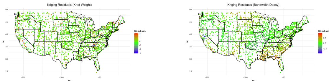
Figure 4.10: Residuals for a randomly chosen weight coefficient (left) and a randomly chosen bandwidth decay coefficient (right) for localized (non-stationary) kriging.
